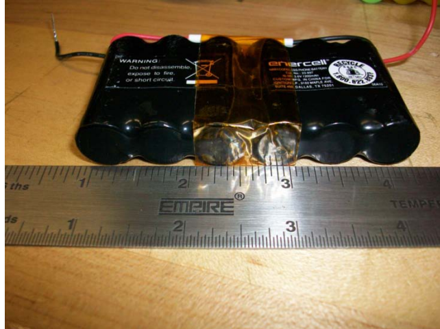
Figure 34 Internal NiMH Battery
